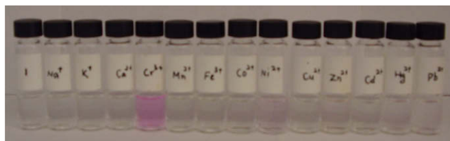
Figure 5. A photograph of compound 1 (10 \mu M) with different metal ions (6 \mu M), from left to right: 1 free, \text{Na}^+ , \text{K}^+ , \text{Ca}^{2+} , \text{Cr}^{3+} , \text{Mn}^{2+} , \text{Fe}^{3+} , \text{Co}^{2+} , \text{Ni}^{2+} , \text{Cu}^{2+} , \text{Zn}^{2+} , \text{Cd}^{2+} , \text{Hg}^{2+} , and \text{Pb}^{2+} .
